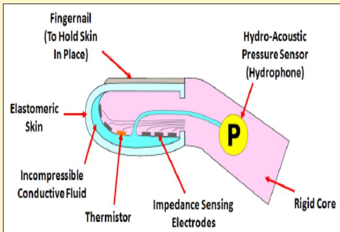
This type of sensor can sense load anywhere and in constraints as a skin sensor. The skin sensor generally provides more accurate force measurement at higher bandwidths. If the manipulator link is defined generally, and the signal point contact is assumed, then the force/torque sensor can give the information about the contact location of force and moments it is called as an intrinsic tactile sensing.
