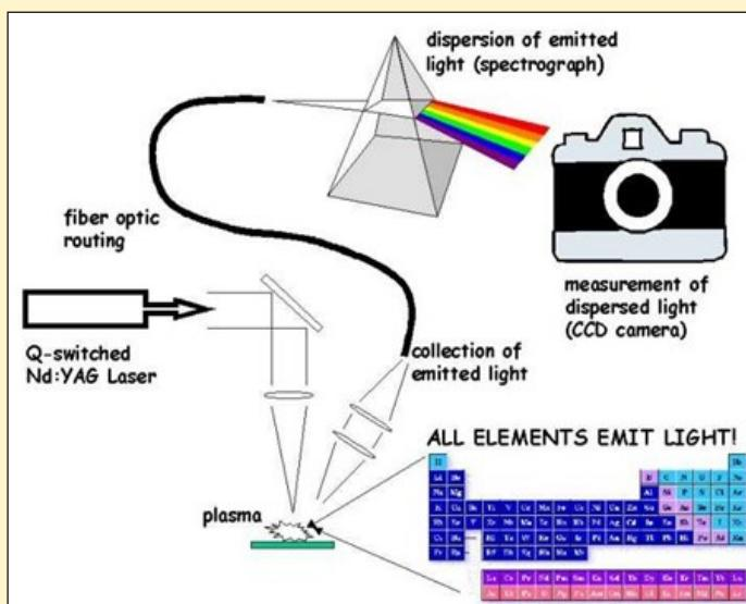
This laser causing a high temperature plasma on the surface of the sample and the light generated indicates composition of the sample. This is a point-and-shoot process that provides fast and accurate results.
